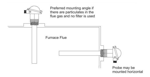
Figure 3-1: Oxygen Probe Mounting
